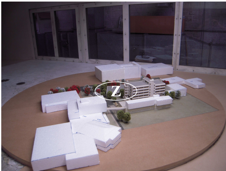
Figure 3.36: 1:200 scale model of building Z and surrounding.
